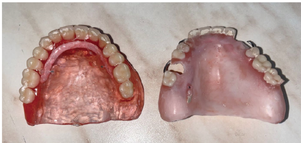
Figure 3: Prostheses produced on the basis of pure (a) and unwashed (b) PMMA.
